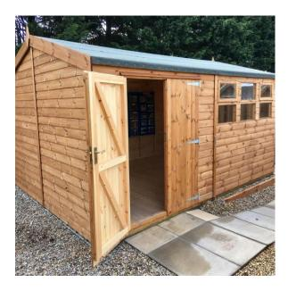
The structure is raised for the purpose of drainage and pest control. The double doors will allow wheelchair access, and HAHA will construct an appropriate ramp. The windows will be made of Perspex, to the specification of HAHA.
